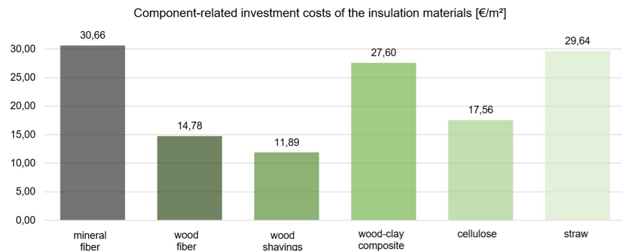
Fig. 2: Economic comparison of component-specific investment costs for insulation materials in €/m² [Saint Gobain, 2025; Steico, 2025; Baufritz, 2022, Holz-Lehmhaus, 2022; Sonnenklee, 2025]
