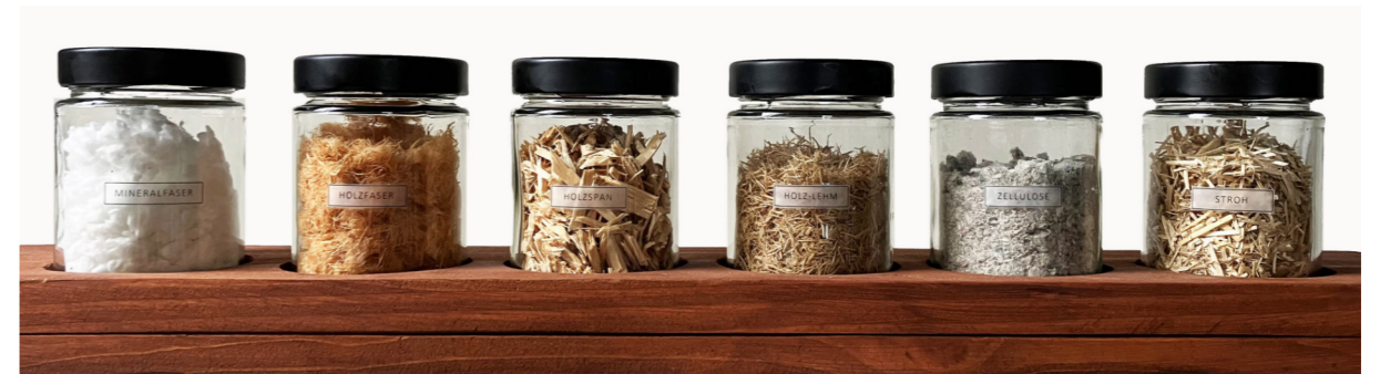
Fig. 1: Samples of insulation materials: mineral fiber, wood fiber, wood shavings, wood-clay composite, cellulose, and straw [© Widmann]
