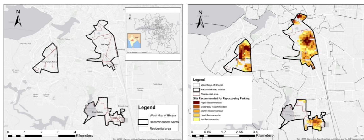
Figure 3: Map showing recommended districts for parking repurposes in Bhopal and results from GIS-based raster analysis identifying optimal sites (Source: Authors)
